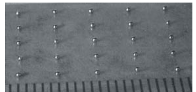
Two samples of tin droplets deposited on steel surfaces which show the repeatability of the process. (Scale in mm)
